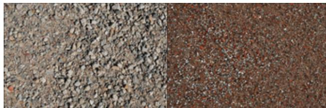
**Figura 9 – (a) Pedrisco (Concreto) (b) Pedrisco (Material Misto)**
