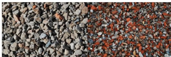
**Figura 8 – (a) Brita 1 (Concreto) (b) Brita 1 (Material Misto)**
